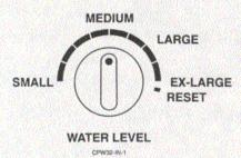
IMPORTANT: Holding the LOAD SIZE (WATER LEVEL) control in the RESET position can cause flooding of the washer.
